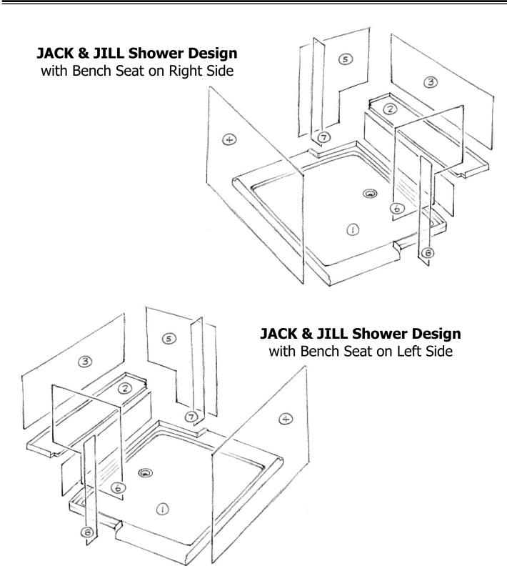
Copy this page, write your dimensions on the copy, and fax to us for a quote. Always give stud-to-stud measurements for base, framing height of bench seat support structure, and distance to top of wall panels from the floor. We will figure clearances etc. Circled numbers indicate assembly order.
