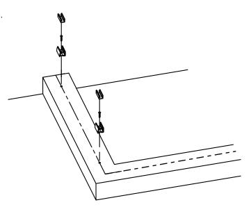
Wall Jamb Installation – Mount the SC-658 Wall Jamb [A] to the return wall.
