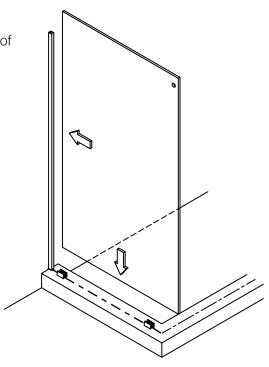
Install the return mount through the hole in the return glass panel. Silicone the gap between the Return Panel [I] and the base curb. Allow the silicone to cure 24 hours before using the shower.
