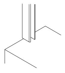
Return Clip Location - Mark the return centerline approximately three inches from the wall and the front centerline. Drill both locations 9/32". Clean the holes and sill of debris, squirt a little silicone into the holes and insert the Glass Clip Anchors [D].
