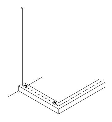
**7** Return Panel Installation – Run a bead of silicone in the center of the the SC-658 Wall Jamb [A]. Then, orient the Glass Return Panel so that the return mount hole is toward the front of the enclosure. Slide the vertical edge of the glass into the siliconed SC-658 wall jamb. Set the bottom edge of the glass into the Glass Clips.
