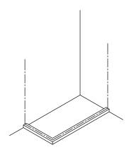
**2** Wall Jamb Installation Preparation – Cut the SC-658 Wall Jamb [A] to the unit height. There may be 3 pre-drilled holes in the Wall Jamb.
