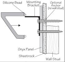
Leave about and 1/8" gap around the edge and the silicone so that it doesn't squeeze out when the shelf is pressed against the wall.
