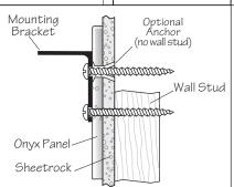
If the screw is not able to hit a wall stud, anchors can be used. Do not over tighten the screw because this may crack the Onyx Panel.
