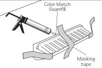
To smooth out a seamfill bead with your finger, dampen a paper towel with rubbing alcohol and then dampen your finger. Next, run your finger along the bead of seamfill, wiping any excess silicone onto the paper towel.
