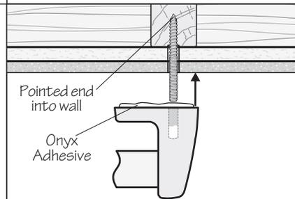
Leaving about 1/8" clean along the edge of the brackets. Do not push so hard that the Adhesive squeezes out from behind the brackets.
