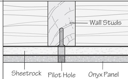
Screw the pointed end into the wall studs or wood backing so that 1" of the bolt remains protruding out from the wall. A good way to do this is to put the bolt in the end of a screw gun, this will help prevent damaging the threads.
