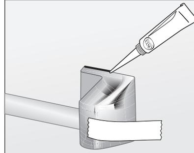
To smooth out a seamfill bead with your finger, dampen a paper towel with rubbing alcohol and then dampen your finger. Next, run your finger along the bead of seamfill, wiping any excess silicone onto the paper towel. The rubbing alcohol will keep the silicone from smearing.
